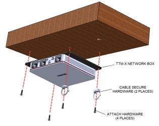
Figure 3 Network Box Installation
